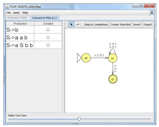
All production rules have been included in the partially complete automaton except for the rules that appear on the left side. For each of these rules (three in the example above), we will create loop transitions around state q1.
